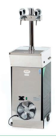
**CWP (Contact Water Power)** – unique construction of the thermal block that combines the advantages of contact cooler and water based cooler in one. The evaporator is in direct contact with the beverage tubing and is able to respond immediately to increase beverage dispensing rate. The time needed to cool the beverage is only 30-40 minutes from turning the device on.
